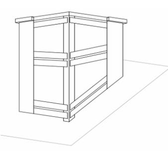
A technical line drawing showing a square roof penetration. The structure consists of a separate understructure (Unterkonstruktion) that supports the cladding (Bekleidung). The cladding is shown as a series of vertical panels meeting at the corners, supported by a frame.               |
