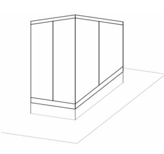
A technical line drawing showing a square roof penetration. The structure consists of a base layer (Unterkonstruktion) and a cladding (Bekleidung) that covers the sides and top of the penetration. The cladding is shown as a series of vertical panels meeting at the corners.             |
