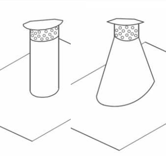
A technical line drawing showing two circular roof penetration details. The first detail is a cylindrical structure with a flat top cover and a seal. The second detail is a conical structure with a flat top cover and a seal. Both details are shown with a circular hole in the center. |
